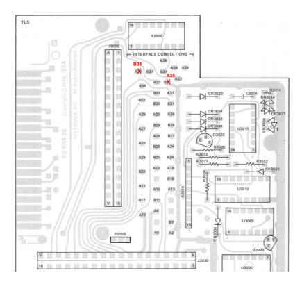
Not noticing this error led many people the wrong way, attempting to cut the ground connection on the transverse board (lifting A35 off ground). The actual grounding of B35 is not on the transverse board, but on the PCB which performs the role of the mainframe vertical slot connector (also explained in "Installation of Option 12 in 7L5 module (S/N  $\geq$  B070000)" document). My recommendation for the spot where ground should be cut is on the following photograph:
