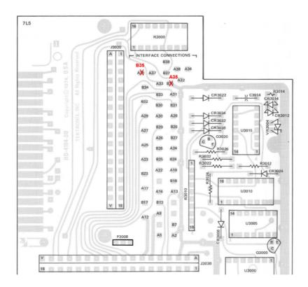
Not noticing this error led many people the wrong way, attempting to cut the ground connection on the transverse board (lifting A35 off ground). The actual grounding of B35 is not on the transverse board, but on the PCB which performs the role of the mainframe vertical slot connector (also explained in "Installation of Option 12 in 7L5 module ( $S/N \ge B070000$ )" document). My recommendation for the spot where ground should be cut is on the following photograph:
