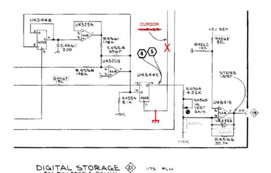
Deletion of cursor is necessary only in digital storage mode, as it's not displayed when digital storage is switched off.
