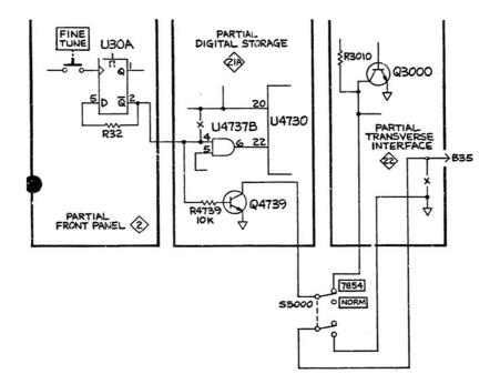
The schematic above also shows the Tektronix recommendation to use the front panel FINE button to switch the modification on or off. Here Q4739 is added to pull the Q3000 collector low, deleting the marker. This implementation makes the instrument start up with modification switched on (as FINE is normally off after power on). A recommendation on how to connect this is in the last chapter.
