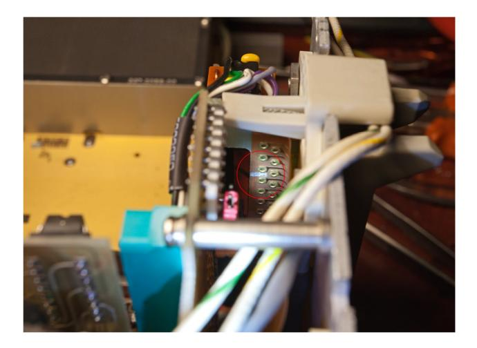
Transverse board and connector PCB (both classic FR4 material) are connected using the polyimide flexible flat cable (brown/orange color), where rivets are used for both electrical contact and mechanical coupling. The ground track that needs to be cut is actually under the polyimide, on the connector PCB (see red circle on the photo above). A small rectangular cut can safely be made on the polyimide here, and the track underneath between the rivets can be severed.
